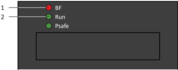
Ilustr. 66: Diody LED stanu PROFINET
