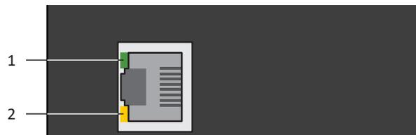
Fig. 89: LEDs for the state of the service network connection
