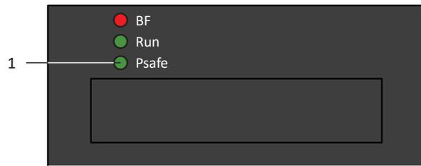
Fig. 87: LEDs for the PROFIsafe status
