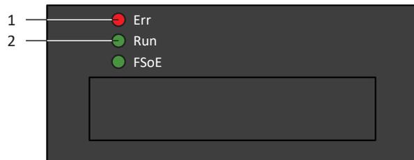
Fig. 84: LEDs for the EtherCAT state
