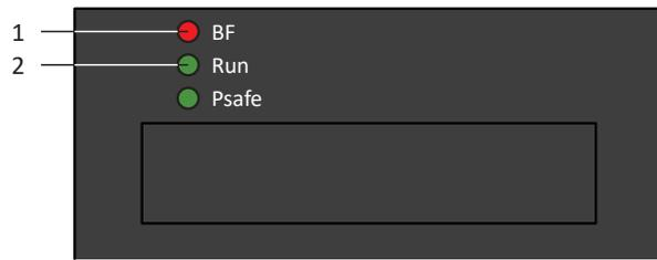
Fig. 86: LEDs for the PROFINET state
