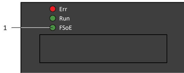
Fig. 85: LED for the FSoE state
