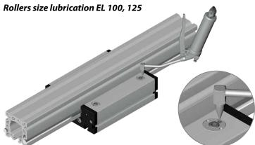
Rollers should be greased each 1.000 working hours or each 6 months with a grease gun. For greaser nipple look at the eccentric at carriage bottom. Use roller grease.
