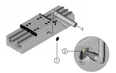
Runner blocks have to be regreased with high quality bearing grease.
