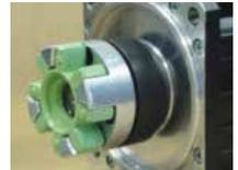
With the coupling and insert installed, guide the motor shaft into the gearhead brake. Support the gearhead during installation as some maneuvering may be required to attain correct alignment with the brake coupling.
