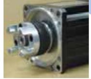
To secure the coupling use a torque wrench to tighten the three (3) allen head screws to the recommended torque in Table 1.
