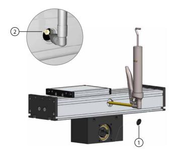
Lubrication is effected by an oiled felt insert. The felt can be re-oiled through lubrication nipples attached laterally to the ends of the roller packs.
