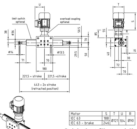
Stroke length up to 500 mm on each side
