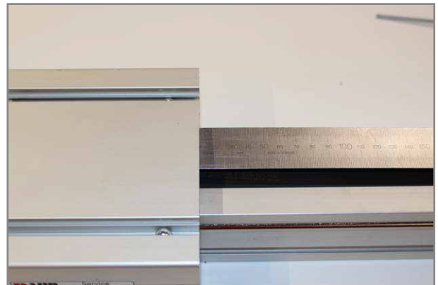
Measure and record the screwing depth on the fastening screws of the toothed belt tensioner.
