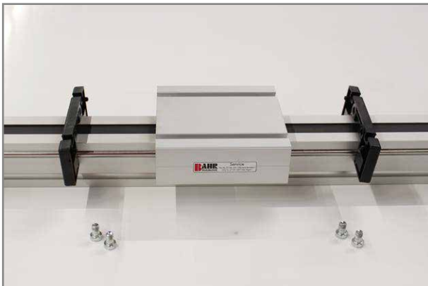
Dismount wiper end plates on both sides of the carriage. Take care, that the felt wipers don't drop out!
