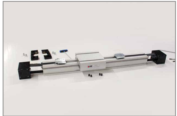
Separate the bearing blocks from the unit.
