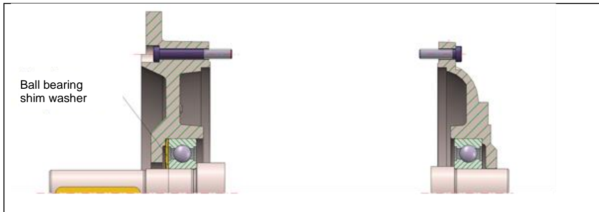
Fig. 1: Constructional design of bearings sizes 63-112
