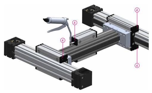
Rods will be greased by the strippers of carriage. There are 2 oil nipples in each wiper end plate (4), where the tanks for the strippers can be filled with an oil gun.
