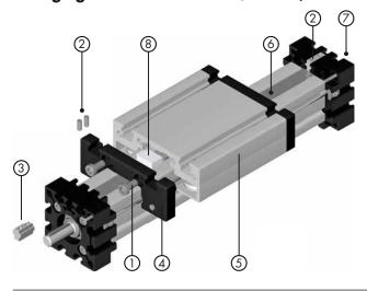
Rollers should be greased each 1.000 working hours or each 6 months with a grease gun. For greaser nipple look at the eccentric at carriage bottom. Use roller grease.
