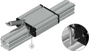
Rods will be greased by the strippers of carriage. There are 2 oil nipples in each wiper end plate (4), where the tanks for the strippers can be filled with an oil gun.
