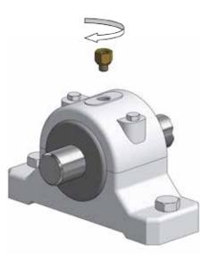
**4.** Lubrication point, accessory parts and tubes must be pre-filled with lubricant. This enables the lubricant to immediately reach the lubrication point.
