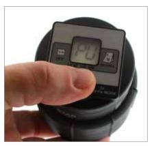
**10.** If counter pressure doesn't decrease you need to either select a different lubricant or a different lubricator. Please ask perma-tec to assist you in this matter
