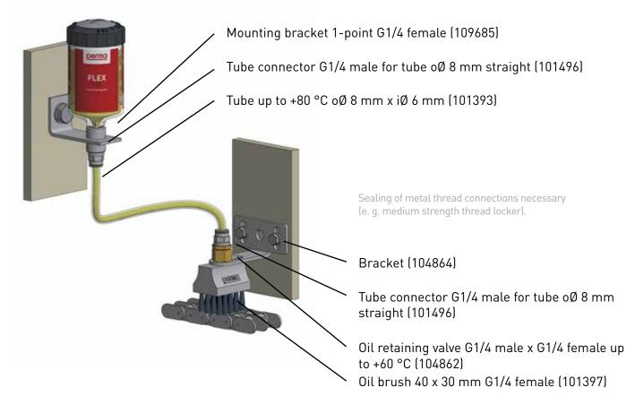
**1.** Prior to installation, lubrication point must be cleaned to protect against contamination.
