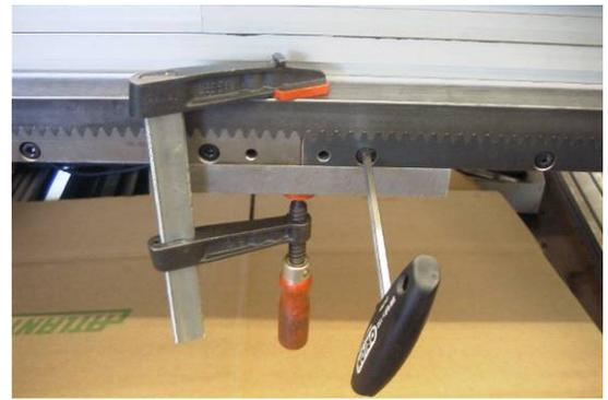
☺ Mounting example on the machine bed
