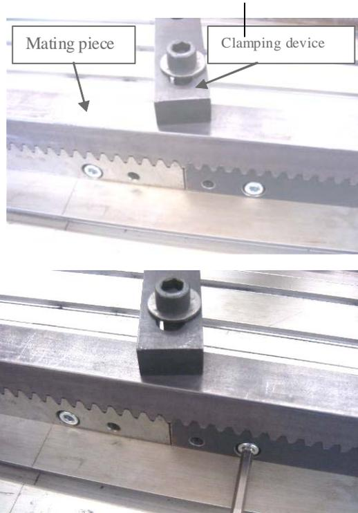
2. Insert the mating companion piece over the joint so that it meshes with the teeth of the two racks and clamp it with a suitable clamping device on the supporting surface.
