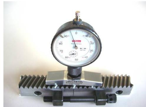
7. Using a hexagon socket wrench adjust the set-screw of the displacing unit in such a way that the rack, which is not yet firmly screwed, can be moved to the left or the right until the dial gauge reaches the zero position again.
