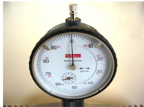
6. Plug the displacement unit into the pinholes at the joint of the two racks. One measuring roll is laid into the tooth gap at the joint and the other two in a tooth gap left and right of the joint. Position the measuring bridge on the rolls so that the feeler of the dial gauge can feel the medium roll. Now seek the zero point by displacing sideways.
